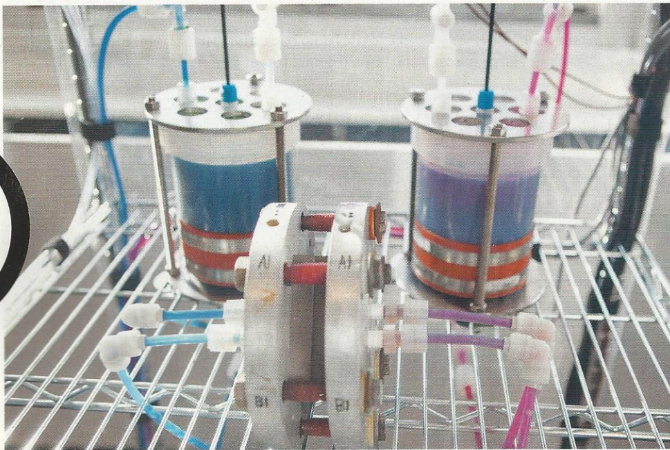
A prototype metal-free flow battery developed by engineer Michael Aziz (bottom) and colleagues at Harvard University relies on the electrochemistry of naturally abundant, small organic molecules to store electricity generated from renewable, intermittent energy sources.
