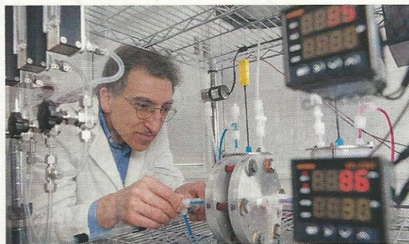
Aziz's prototype would cost much less than other flow batteries.
