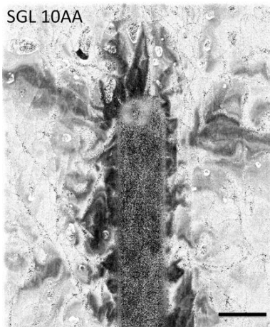
Figure 6. Fluorescence microscope image of the IDFF inlet channel end distributing oxidized AQDS into SGL 10AA carbon paper. Fluid flow and reduction current are constant. The dark regions are areas of more rapidly-refreshing AQDS and suggest pathways of lower pressure drops. Scale bar is 1 mm.
