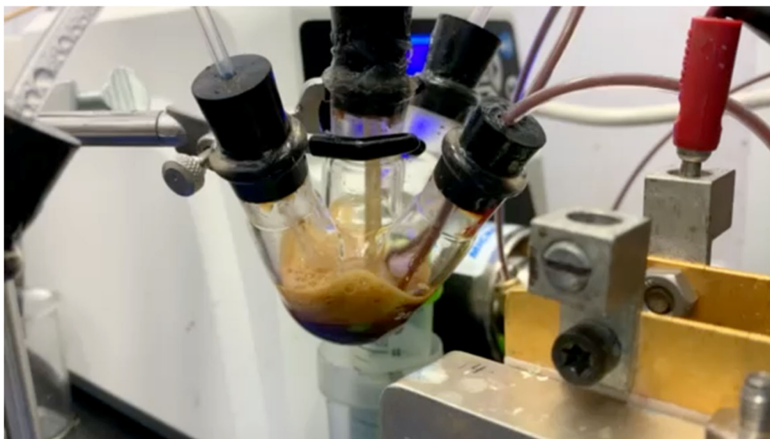
Supplementary Fig. 23 | Cycling of 0.1 M DSPZ under 10 % CO 2 and 90% N 2 . Significant foaming was observed.
