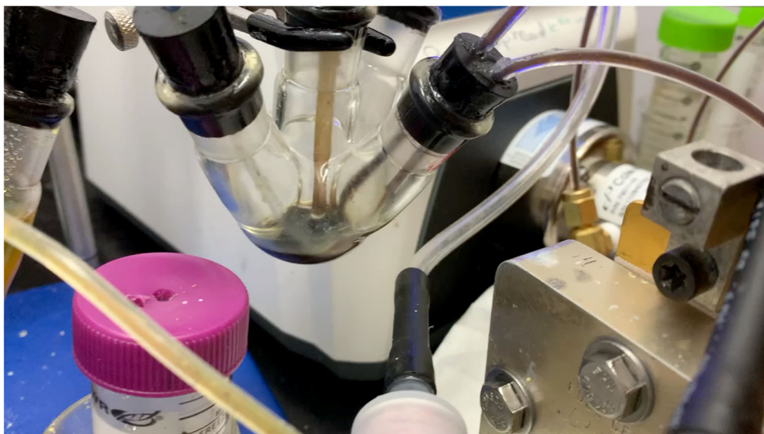
Supplementary Fig. 24 | Cycling of 0.5 M 1,8-ESP under 10 % CO 2 and 90% N 2 . No foaming was observed.
