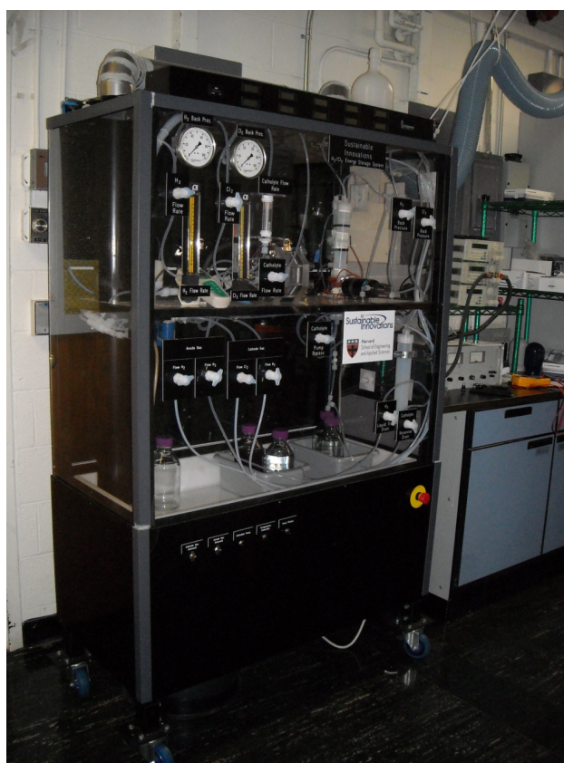
Fig. 3 Image of the test bench used for cell tests. The entire cavity of the bench is held under negative pressure for safety reasons.
