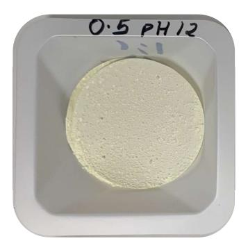
Figure S3: Photograph of example filter paper used to filter precipitates from a saturated solution of ferrocyanide with mixed sodium and potassium counterions and then dried in air. The mass of the precipitates was used to determine horizontal error bars in Figure 6 of the main text.
