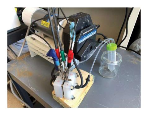
Figure S2: Photograph of assembled flow cell with electrolyte circulated on both sides from a single reservoir, using a Masterflex peristaltic pump. The clips connect the cell to a Gamry Reference 3000 potentiostat.
