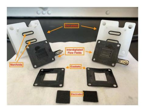
Figure S1: Photograph of the flow cell hardware used for determining membrane conductivity, showing plastic end plates, manifolds, graphite interdigitated flow fields, gaskets (2.55 cm<sup>2</sup> windows), and Sigracet GDL 39AA electrodes.
